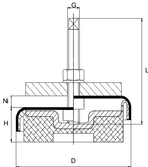
**Construction** Rubber NBR 80 Sh A or 65 Sh A
