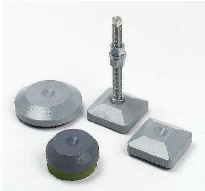
**Construction** Painted cast iron cup with central housing for positioning a precision leveling screw and gluing a high damping capacity VIBRADAMP elastomer
