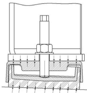
LMPS have the advantage of combining static and dynamic forces at the same central point. The forces are distributed via the internal plate on the elastomer thus ensuring a better distribution of the stress.
