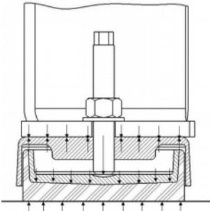
The pivoting effect of the cup also makes it possible to distribute the forces because it is rare for a floor to be perfectly flat. As the stress is better distributed the life of the isolator is improved, stability builds up and better Vibration isolation is achieved.
