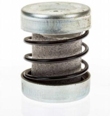
**Materials** Spring with Shot peeling treatment to improve its dynamic resistance and epoxy finish for better protection. Polyethylene softened with closed cells to prevent the entry of solid elements and avoid any damage to the coils. Zinc plated metal parts
