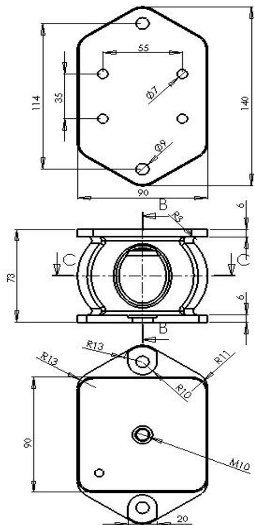
Materials      Rubber NR bonded on 2 steel fixing plate
